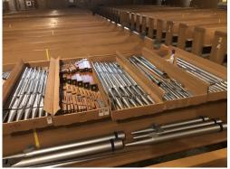
Up to this point about 50% of the Pipes in the Swell Division have this problem. With these pipes being removed due to the cleaning it makes sense to also restore the Swell Division at this time.
